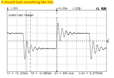
Then use a higher value resistor compared to what you found in step (i) for overdamped response (say 3.3K ohms). Include both LTSpice sims and built circuit response.
